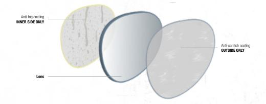
At Bollé Safety Standard Issue, we are convinced that scratches and fog do not only attack specific surfaces. This is why we have decided to permanently apply the anti-scratch AND anti-fog coating to each lens surface (inside AND outside).
